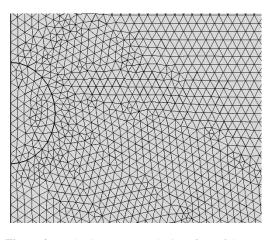
Figure 2. Mesh elements near the interface of the two phases
