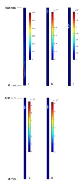
**Figure 5**. Velocity fields [m/s] in case of the different fluids. a) water, b) silicone oil, c) paraffin oil 1, d) paraffin oil 2, e) gear oil
