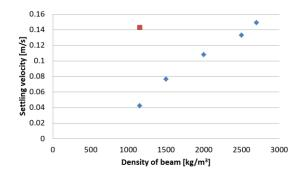
**Figure 3.**Settling velocities of different density bead (blue diamond) and the measured velocity (red square)
