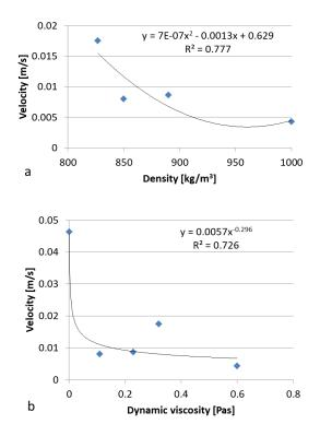
Figure 7. Diagrams of the density (a) and viscosity (b) dependence of velocity
