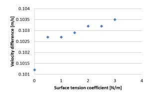
Figure 4.Effect of surface tension coefficient on the error of the simulation compared to the measurement
