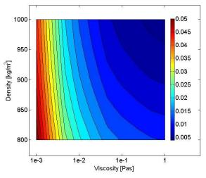
Figure 8. Velocity [m/s] as a color map in dependency of density and viscosity of Fluid 2
