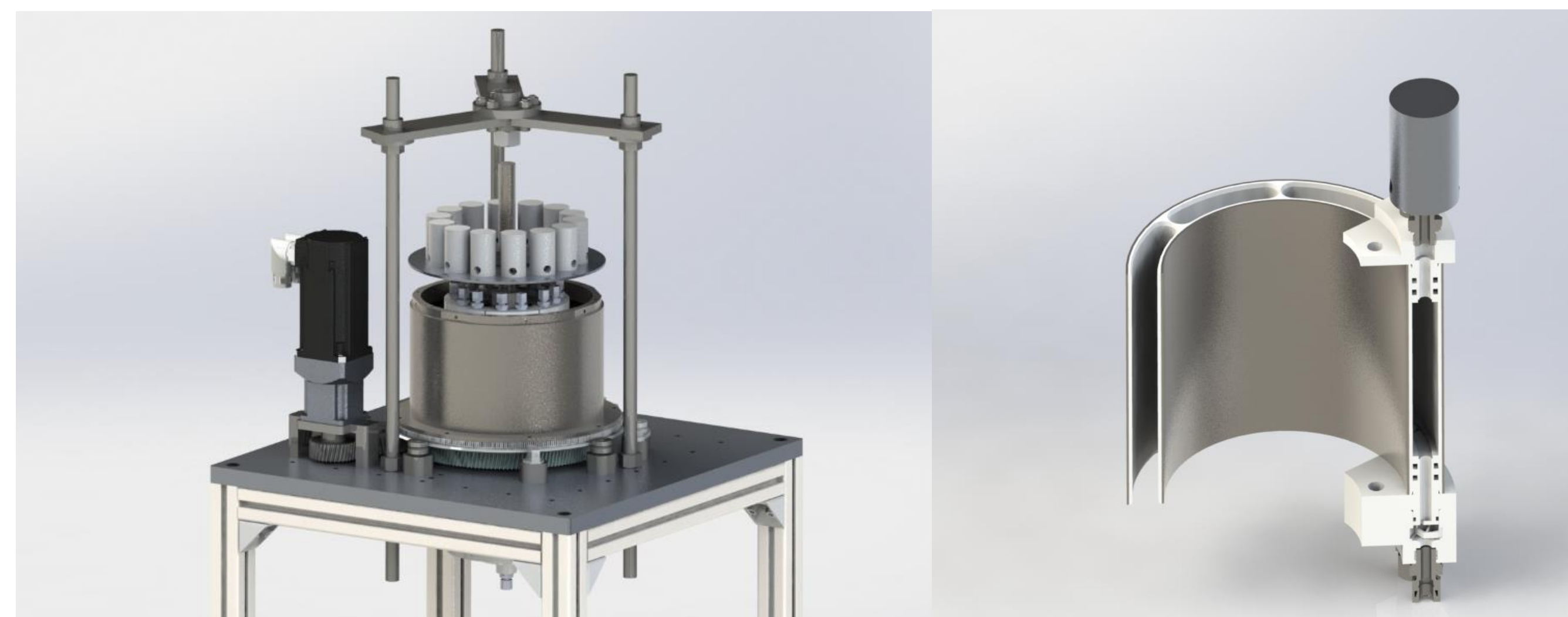
Fig.1 Magnetic refrigerator system and AMRs with valves
