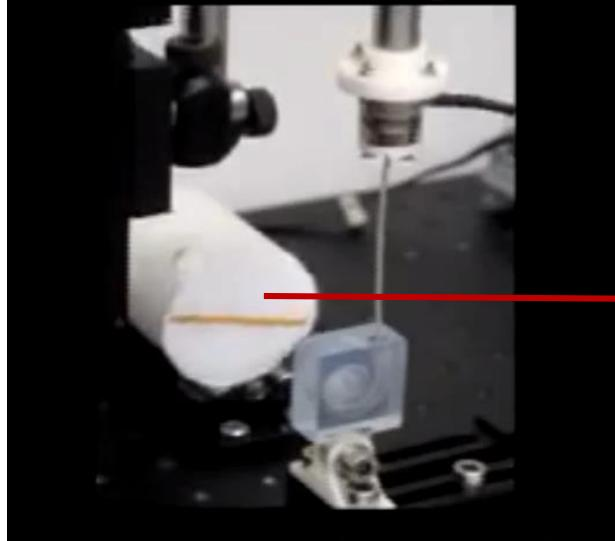
Magnet that guides the cochlear implant electrode array
