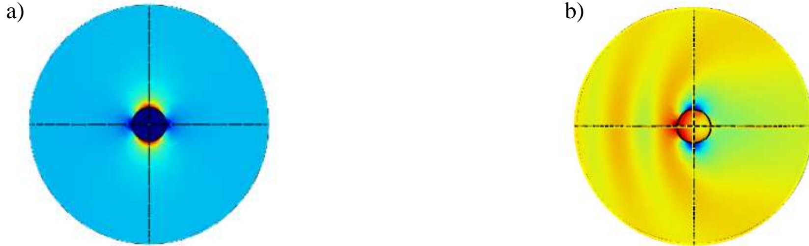
Figure 6. Distribution of scattered electric field for Teflon of a) 20 \mu\text{m} and, b) 100 \mu\text{m} radius at different frequencies.
