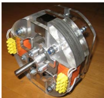
Figure 13. Switchable PPMT motor (the prototype).
