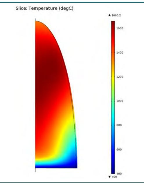
NUMERICAL MODELING OF COLD CRUCIBLE INDUCTION MELTING
