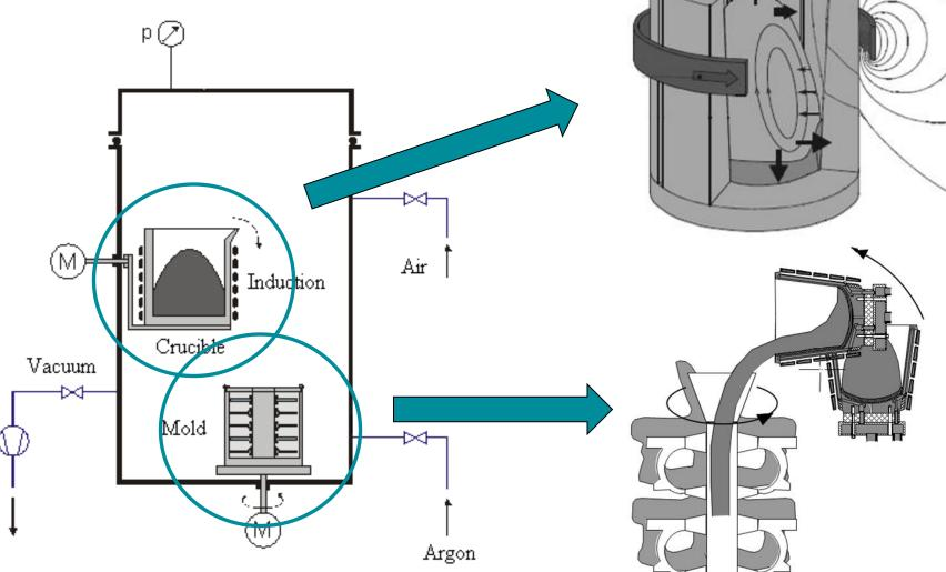
NUMERICAL MODELING OF COLD CRUCIBLE INDUCTION MELTING
