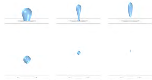
Figure 6. 3D, 1/8 -symmetry model of a single vapor bubble.
