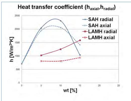
Figure 9. Heat transfer coefficients between the hot disk and the sample.
