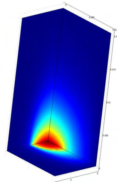
**Figure 3.** Solution of the forward problem after 5 seconds of heating. Only ¼ of the physical domain has been modeled.
