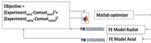
**Figure 4.** Schematics of interaction between Matlab optimizer and solving the backward problem and Comsol solving the forward problem.
