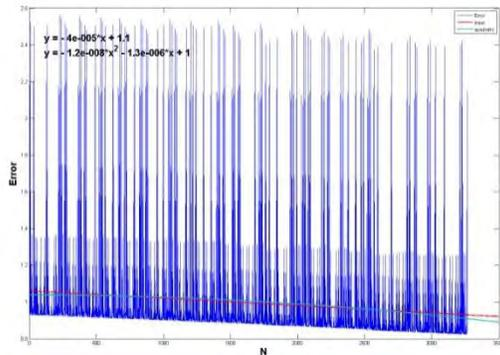
**Figure 6.** Dynamics of objective function drop in course of *patternsearch* work parameterized with the number of steps. The size to the leap step in terms of the number of the *patternsearch* steps is determined by requesting the desired drop of the objective function. Note that requesting zero value is not the best choice as the minimum could be missed. The optimal value is determined by the line search along the smoothed parameter manifold parameterized by the *patternsearch* steps.
