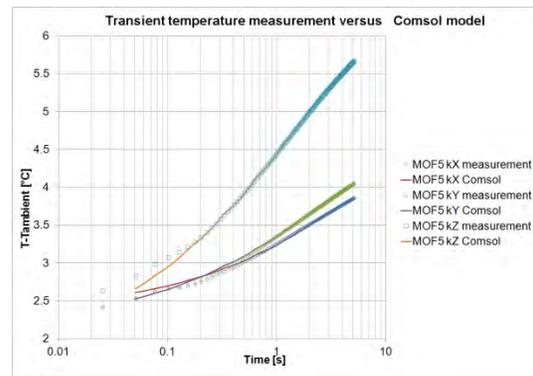
Figure 11. Experimental measurements versus Cmsol inverse problem solution for MOF5 compound when three time traces of measurements in all perpendicular directions have been used in objective function.
