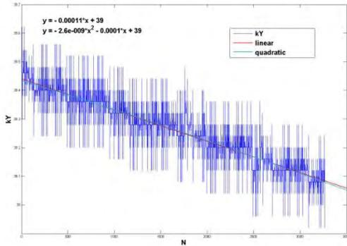
**Figure 5.** Typical dynamics of a parameter change in course of *patternsearch* work parameterized with the number of steps.
