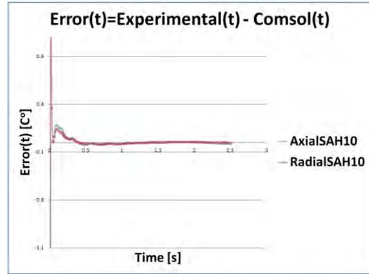
Figure 10. The difference between Cmsol model and experimental measurements.
