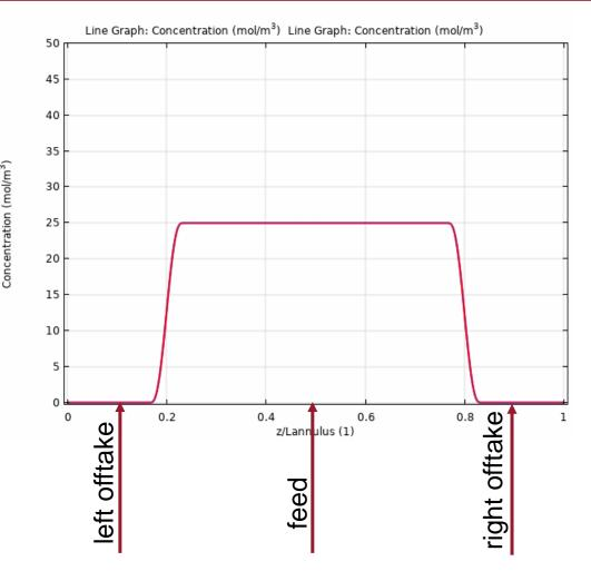
COMSOL Multiphysics<sup>®</sup> simulation of the evolution of a separation of two species with 0.25% difference in their electrophoretic mobilities in a 12-inch wide recycle CFE. Feed is continuously injected into the bottom center port and products are taken out of the chamber at the left and right offtake ports. Recycling allows the hold-up time to be increased until the two species are separated.
