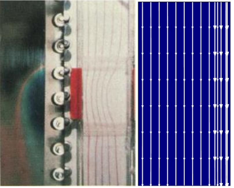
COMSOL Multiphysics<sup>®</sup> simulation of the flow instability in a continuous flow electrophoresis apparatus. This instability, which manifests as an asymmetric vortex attached to one side of the chamber, can be greatly reduced by using upward flow and insulating the heat-transfer surfaces on the front and/or back surfaces.
