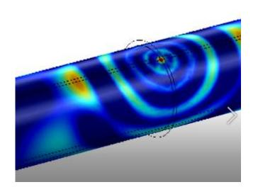
"Investigations found that the dominant mode that propagates over significant distances in buried water mains is a mode which at low frequencies is characterized by predominantly axial water-borne displacements. The established method of locating leaks by acoustic signal analysis assumes that leak noise propagates as a single non-dispersive mode at a velocity related to the low frequency asymptote of this water-borne mode."
